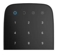
When touching KeyPad, it wakes up highlighting the keyboard and indicating the security mode: Armed, Disarmed, or Night Mode. The security mode is always actual, regardless of the control device that was used to change it (the key fob or app).
